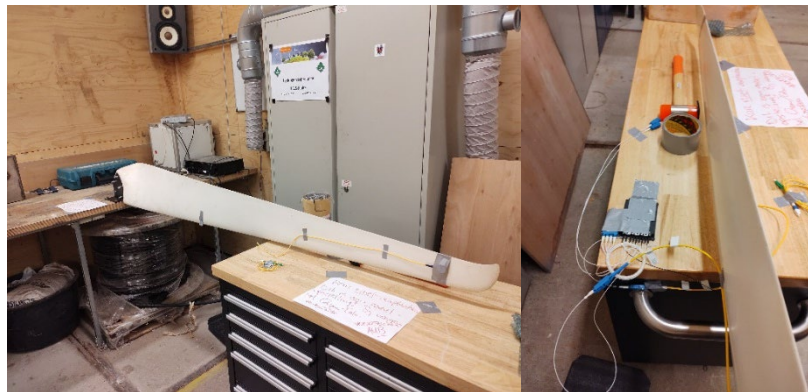
Figure 2: test set up with wind turbine blade and photonic sensors
